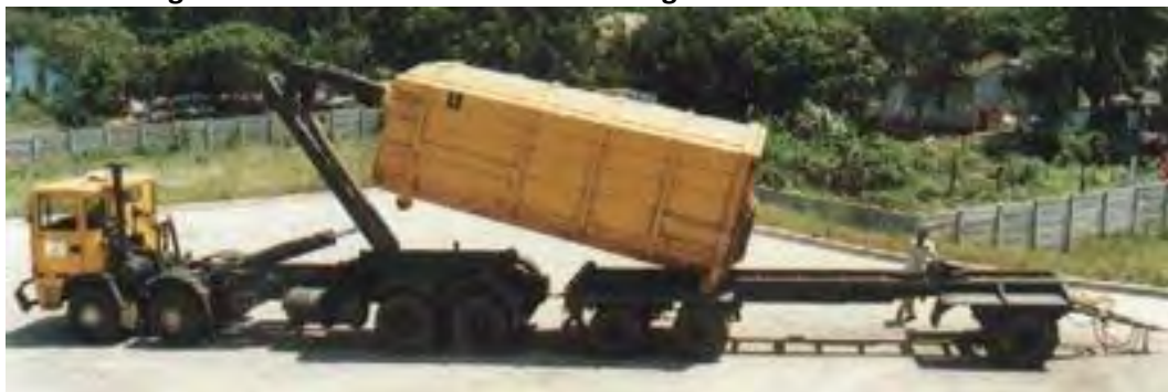
Figure 3-60: Roll-on vehicle transferring full container onto trailer
