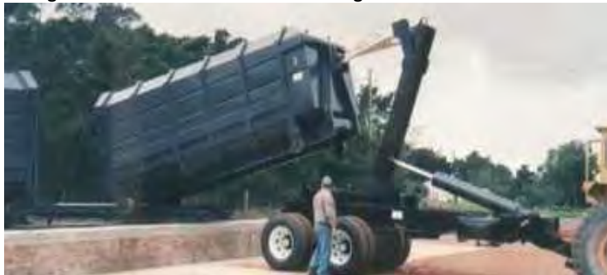
Figure 3-61: Roll-on vehicle transferring full container onto trailer
