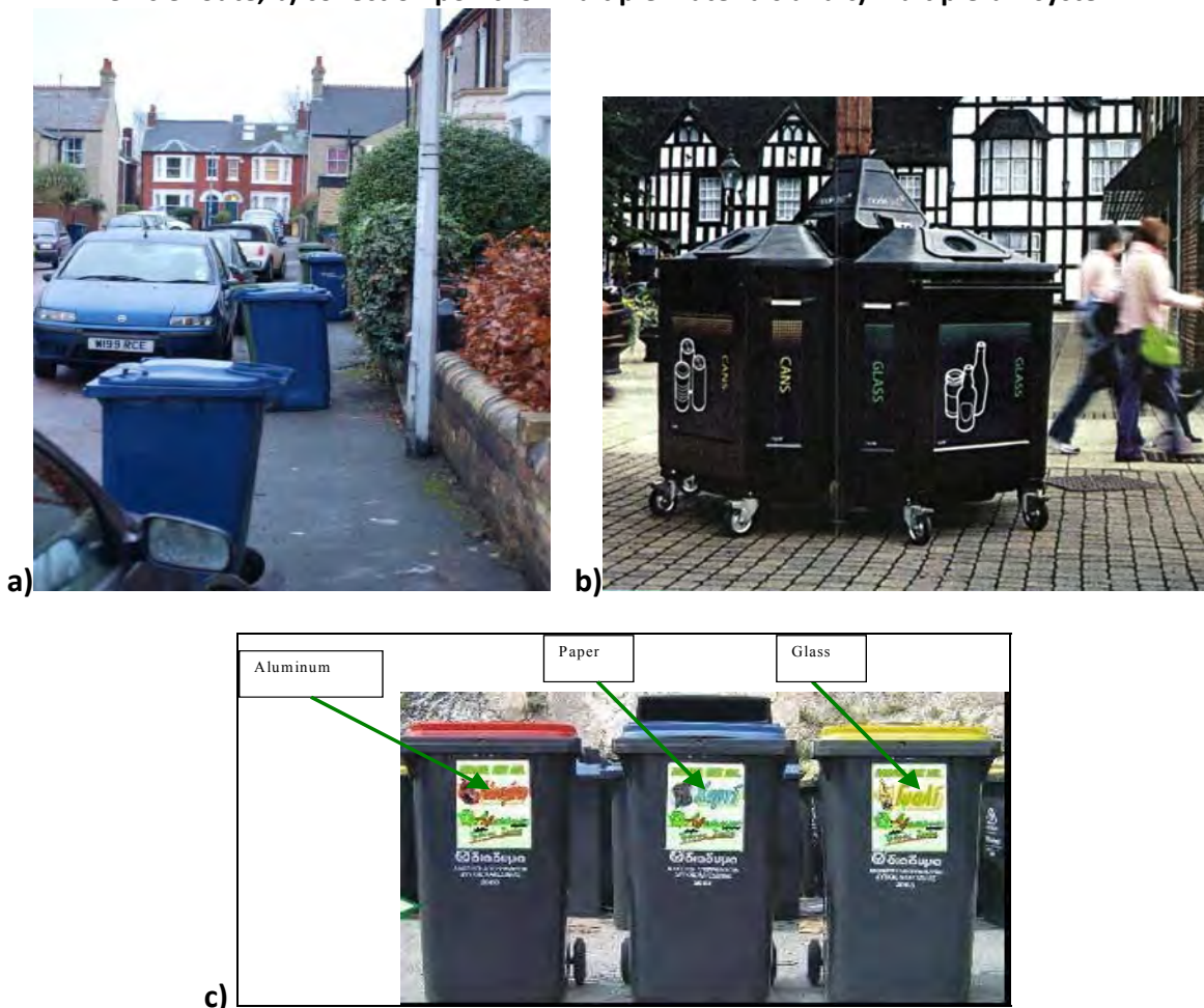
Figure 3-46: Examples of a) door to door collection, where car parking may cause obstruction to the vehicle route, b) collection point for multiple materials and c) multiple bin system
