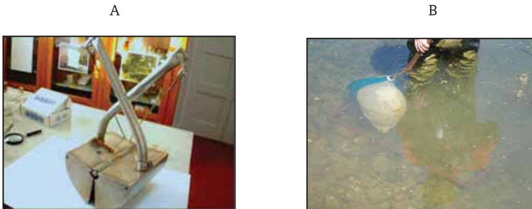
Figure 2. Sampling equipment: van Veen grab and D-shaped net
