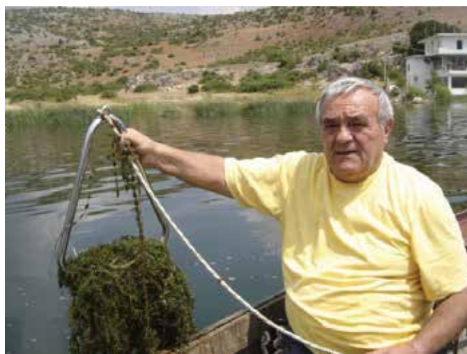
Figure 4: Double-sided Luther-rake used for macrophyte sampling
