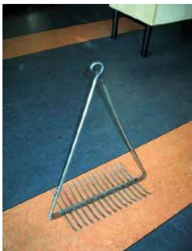
Figure 4: Double-sided Luther-rake used for macrophyte sampling
