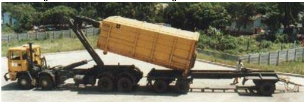
Figure 3-59: Roll-on vehicle transferring full container onto trailer
