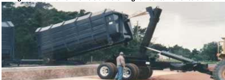
Figure 3-60: Roll-on vehicle transferring full container onto trailer
