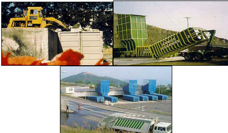
Figure 3-57: Waste disposal in container with no compaction, hopper compaction and automated transfer station
