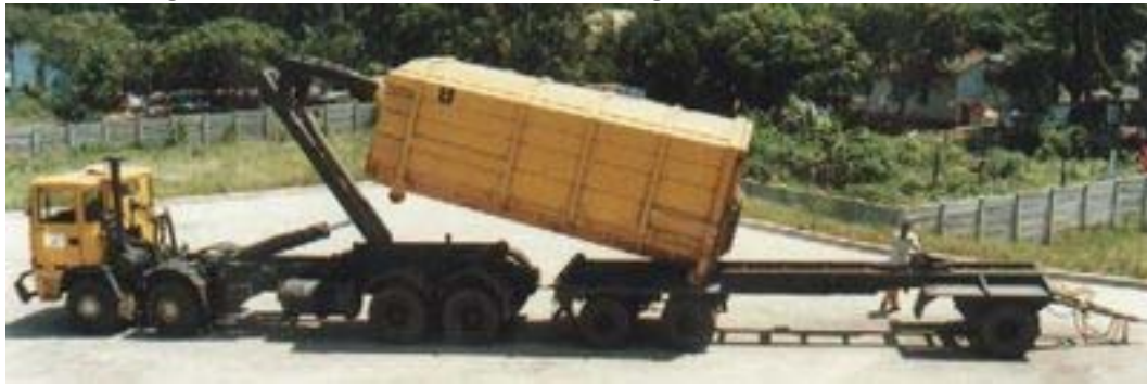
Figure 3-58: Roll-on vehicle transferring full container onto trailer
