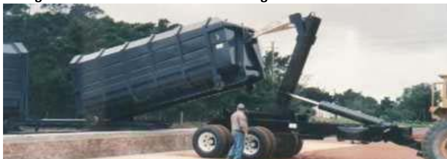
Figure 3-59: Roll-on vehicle transferring full container onto trailer
