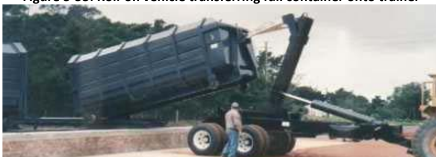
Figure 3-53: Roll-on vehicle transferring full container onto trailer
