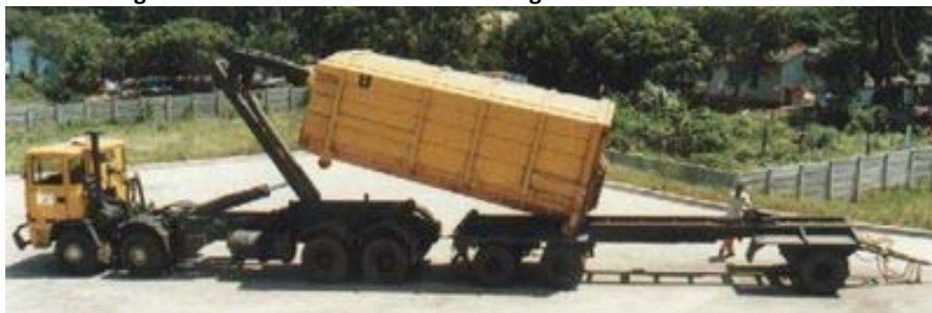
Figure 3-52: Roll-on vehicle transferring full container onto trailer
