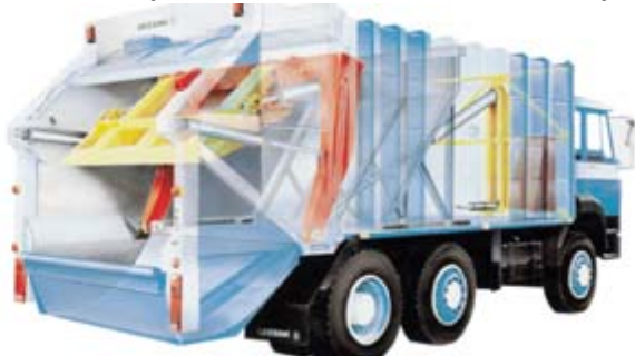
Figure 3-37: Example of a collection truck with compaction
