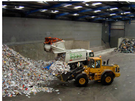
Figure 3-61: Tipping area in Dirty MRF
