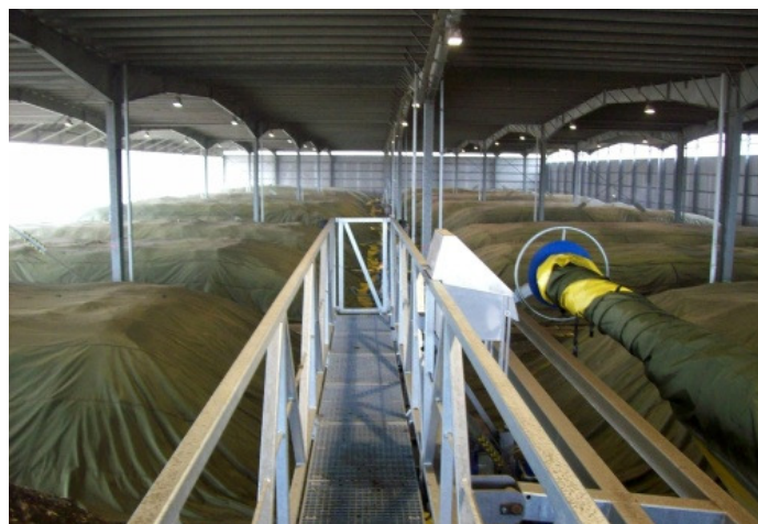
Figure 3-73: Aerated covered heaps (indoors)
