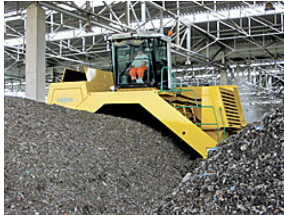
Figure 3-72: Turned windrow compost (Indoors)
