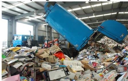
Figure 3-64: Recycling vehicle emptying in Clean MRF
