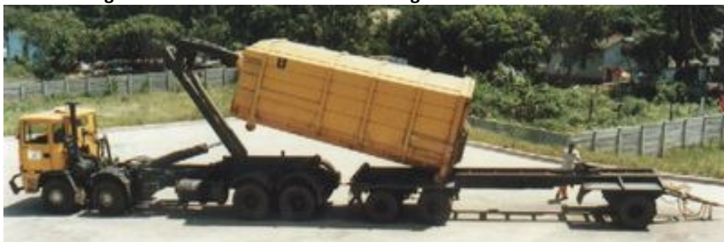
Figure 3-57: Roll-on vehicle transferring full container onto trailer
