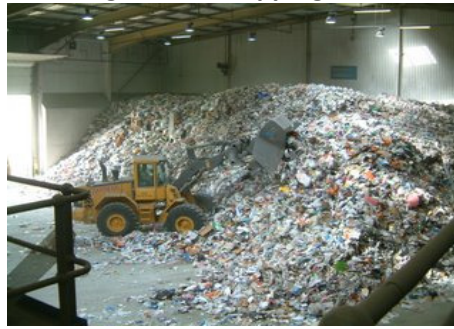
Figure 3-63: Tipping area in Dirty MRF
