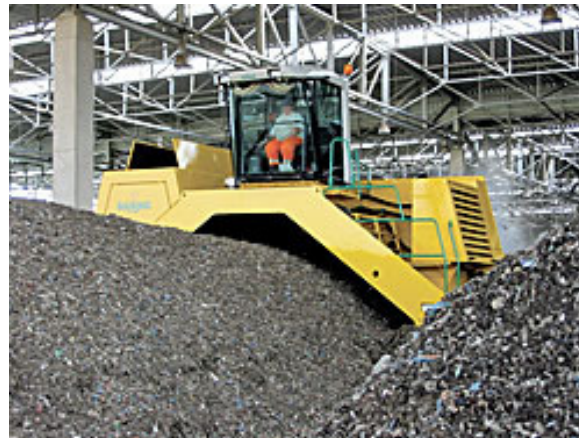
Figure 3-74: Turned windrow compost (Indoors)
