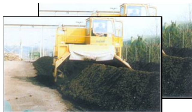
Figure 3-73: Turned windrows compacting system (Open Area)
