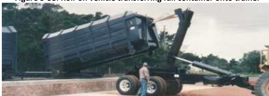
Figure 3-58: Roll-on vehicle transferring full container onto trailer
