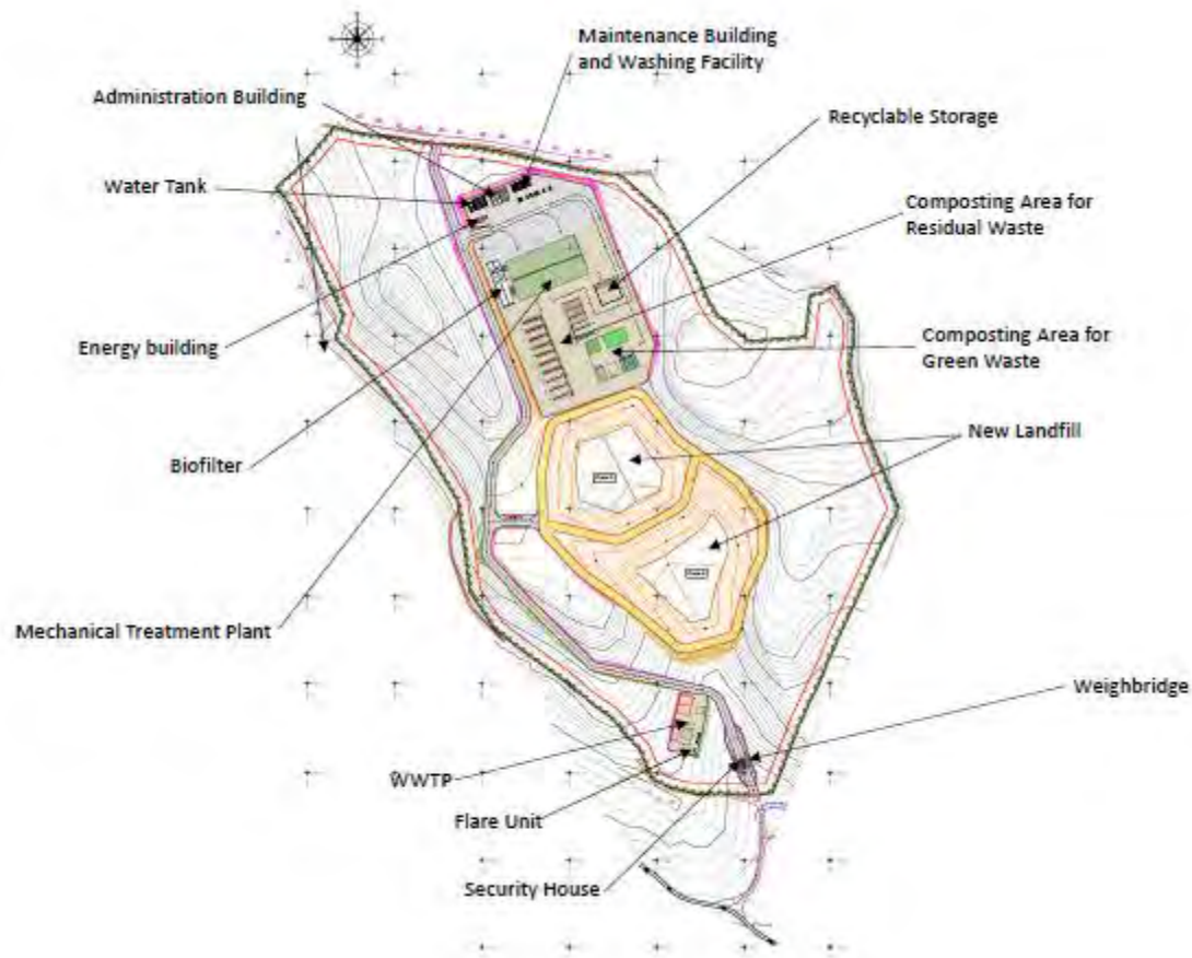
Figure7-58: General layout of Central Waste Management Facilities
