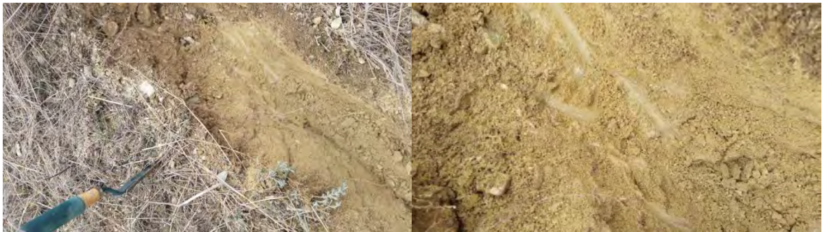
Figure 7-39: Fine granular quartz sands with light yellow colour
