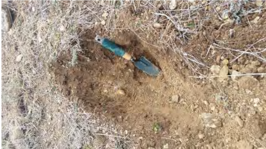
Figure 7-38: Coarse granular (gravel - sandy) sediments with significant amount of clay material
