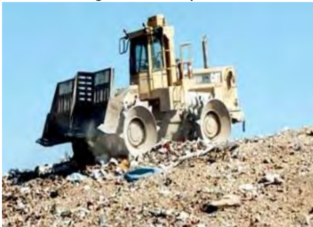
Figure 7-48: Compaction at the landfill and loading of soil cover material
