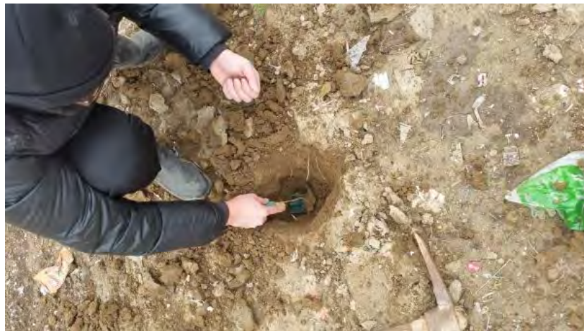
Figure 7-36: Exploration trench located in dusty clays
