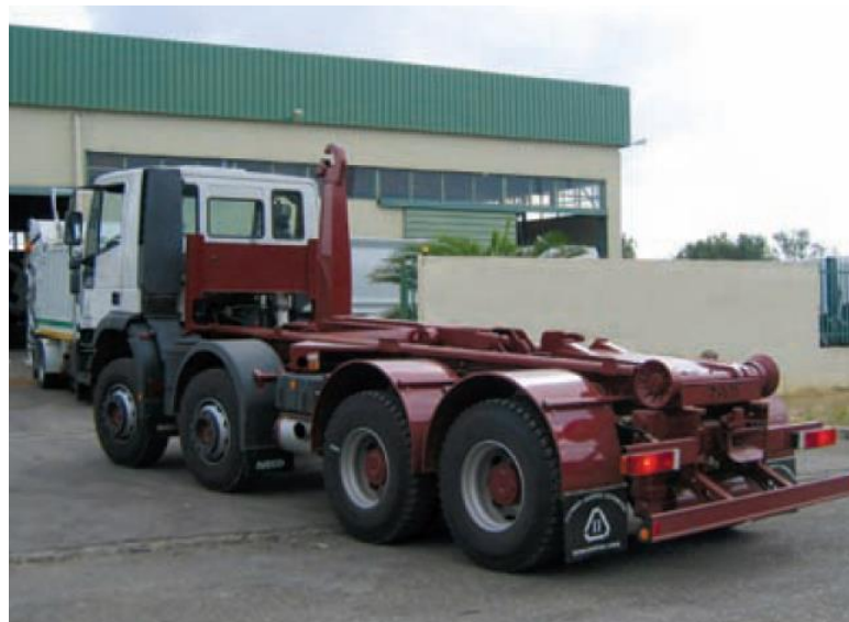
Figure 7-75:Container transport vehicle
