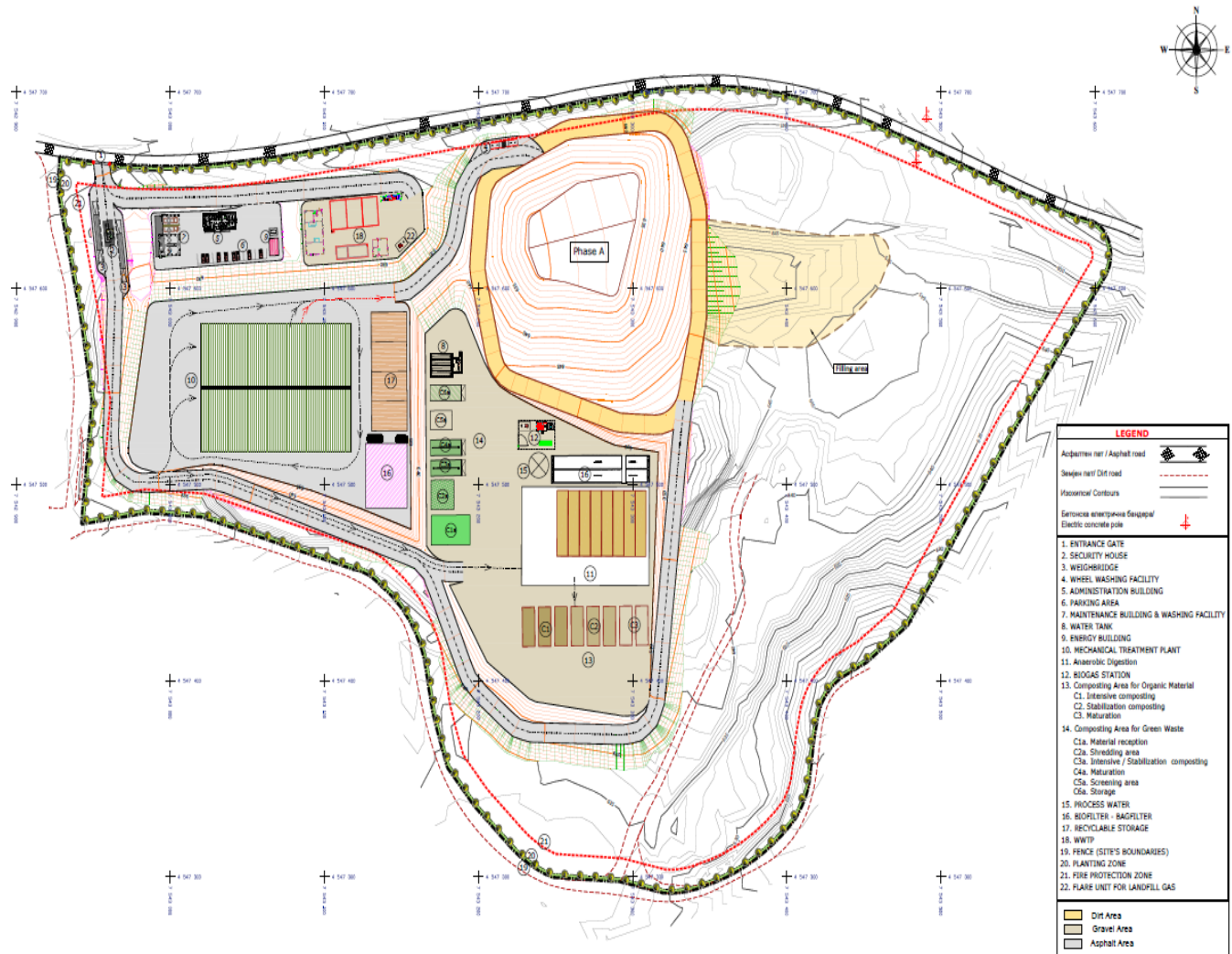
Figure 7-66:General layout of the Waste Management Center (Phase A)
