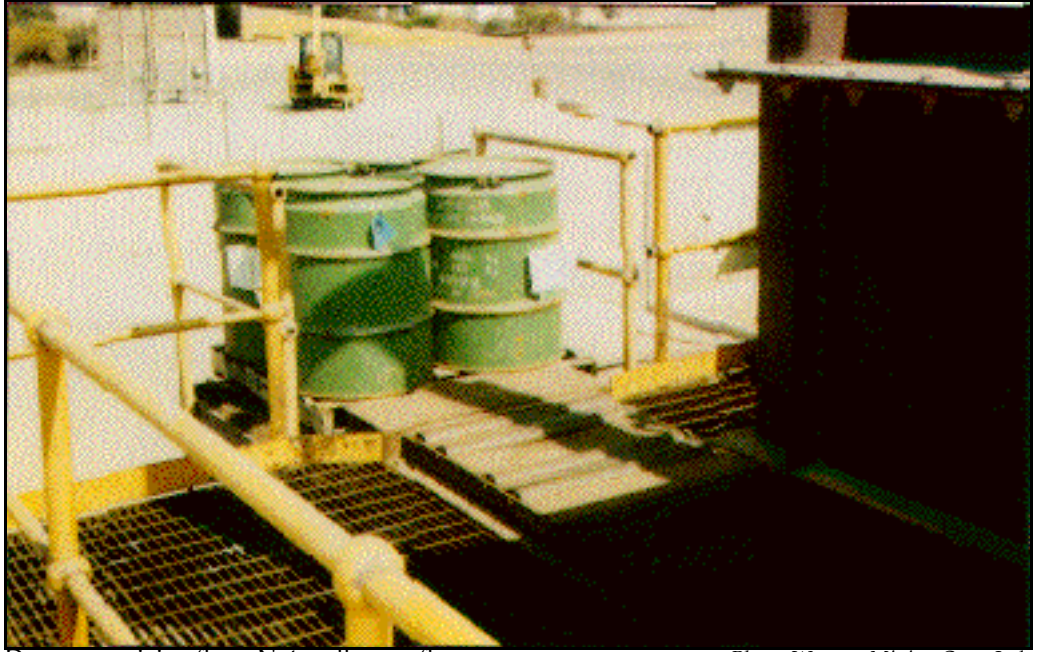
Drums on mixing floor. Note rollers on floor.
